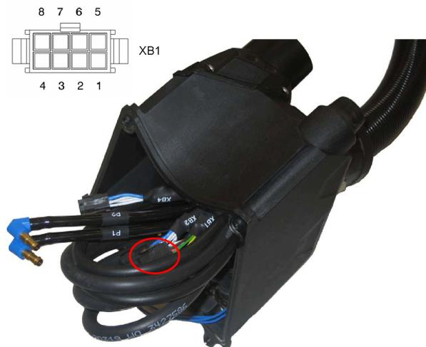
There is a one to one correspondence between the pins of the XB1 and the X1202 connectors.
